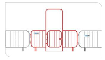
Gated walk through barrier option two is self closing and has a lockable latch.
