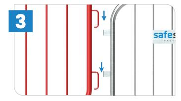
To interlock the barriers, lift the end of the pedestrian up, so that the hook can drop into the hoop on the end of the barrier.
